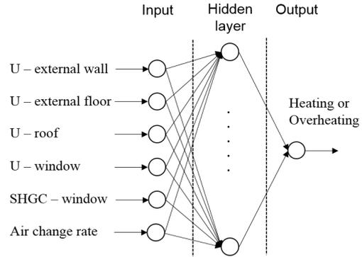
Abbildung 2: Schematic structure of the used neural network
