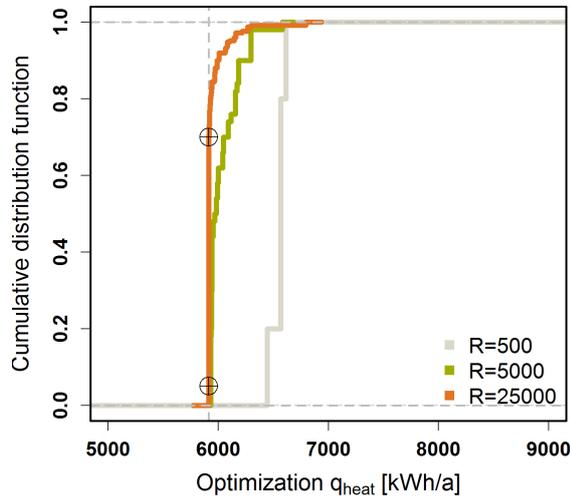
Abbildung 8: Cumulative distribution function of all optimization results depending on the number of runs
