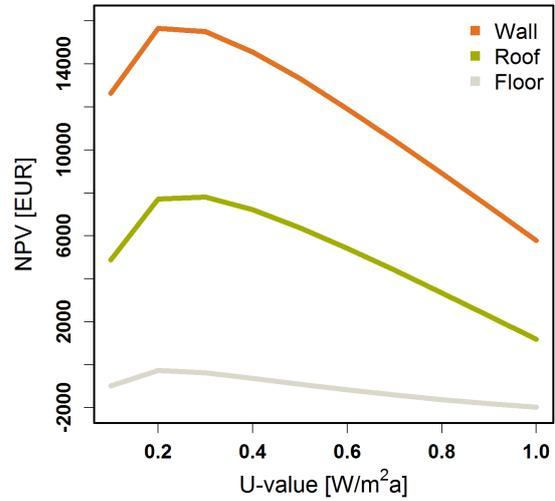
Abbildung 11: Net present value depending on the U-value of different renovation measures
