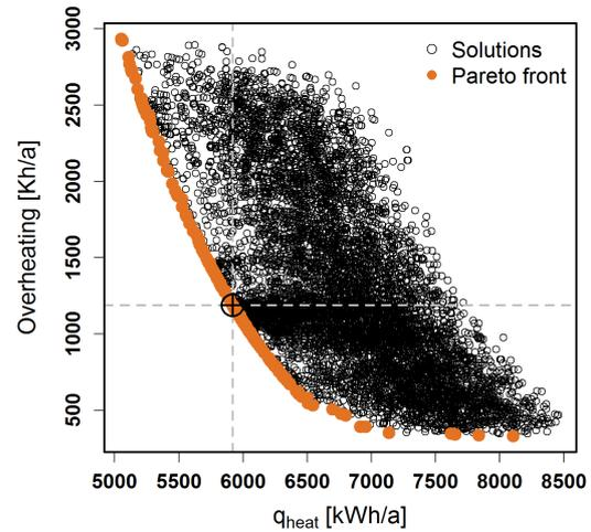
Abbildung 9: Solutions for the optimization of  $q_{heat}$  with a highlighted Pareto-optimal front
