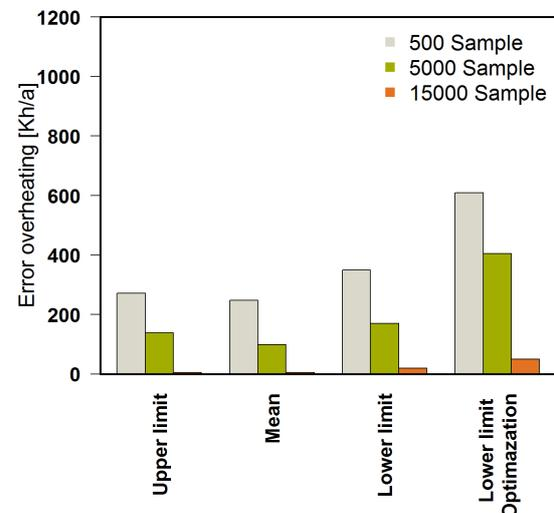
Abbildung 7: Absolute error on the upper and lower limit of the NN-ODH
