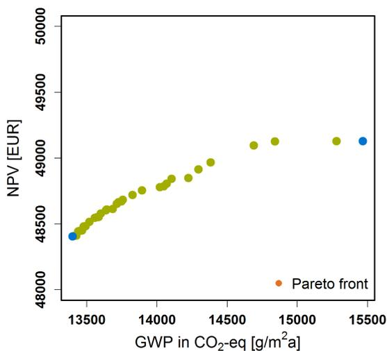
Abbildung 13: Pareto-optimal solutions of the Multi-objective optimization of GWP and NPV
