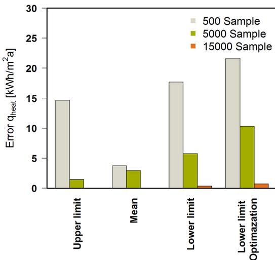
Abbildung 5: Absolute error on the upper and lower limit of the NN- $q_{heat}$
