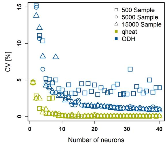
Abbildung 3: Variation of the number of hidden neurons and the influence on the CV for the objectives  $q_{heat}$  and ODH depending on the sample size
